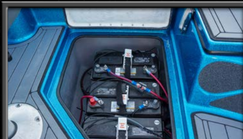
Central battery storage for optimal weight distribution, access, and overall boat control.
