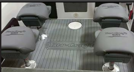
Custom cut foam floor insert for added traction, comfort, and style (standard on 2095 BTX).
