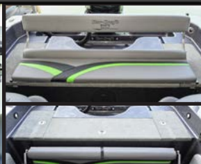
28" or 59" Rear folding bench seat for added passenger comfort.
