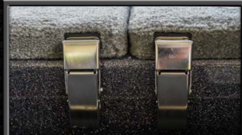
New custom SS livewell latches. Proven to keep lids more secure and livewell water cooler.
