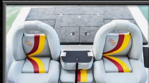
Standard bench seat configuration with a fold down, traction backed seat/step.
