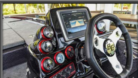
Redesigned console capable of a dual flush mount electronics set up.
