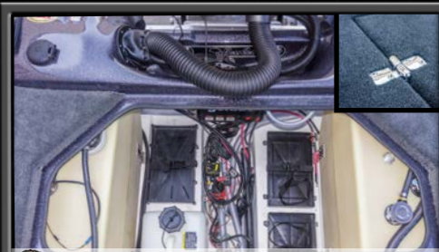
Easy access to pumps, batteries, and fuel. Rear lid can detach (see hinge upper right).
