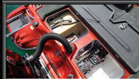
Large bilge, fuel, and battery access. Fold-flat door with detachable hinges.
